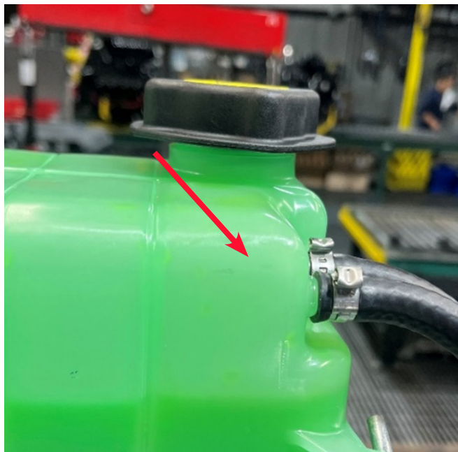
Not Degassing (no coolant flow through vent lines)
