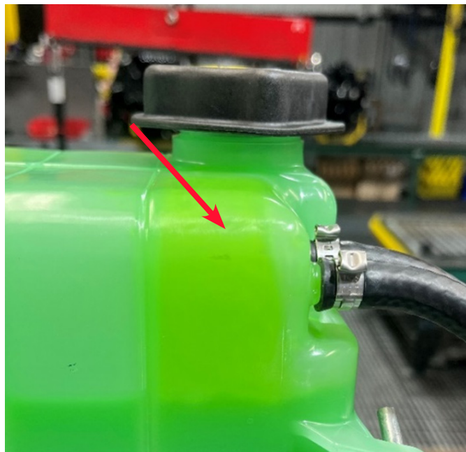
Properly Degassing (coolant flowing through vent lines)
